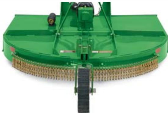
The round-back design allows for easy maneuvering into tight corners and around trees, fences, and other obstacles.
