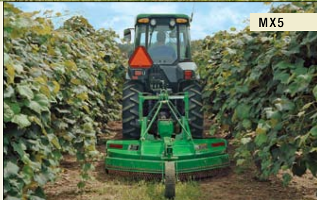
MX5 with 5525 Narrow Tractor cutting between vineyard rows.
