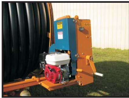
Reliable 5.5HP Gas Mechanical Drive
