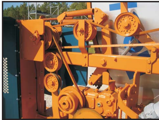
Easily Adjustable Speed Control with 2 Speed gearbox with 2 Step Pulley
